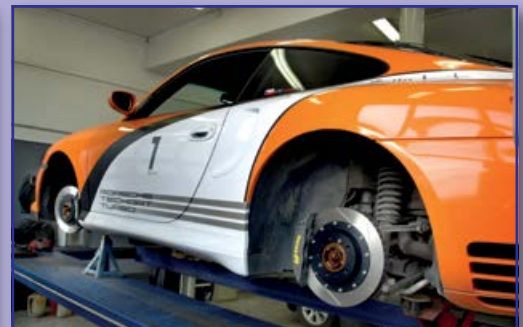
Porsche 911 996 - brake kit for both front and rear axles, parts AP Racing, Wilwood, Rensport
