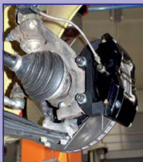
Škoda Fabia RS 1.9 TDI - brake kit for front axle - parts Wilwood, Rensport
