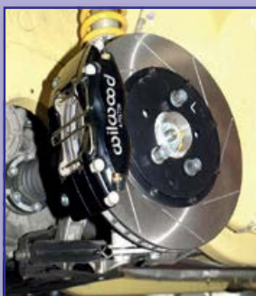
Škoda Fabia RS 1.9 TDI - brake kit for front axle - parts Wilwood, Rensport
