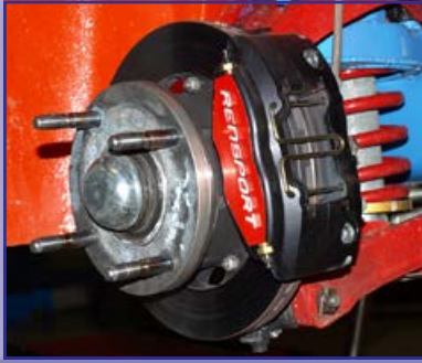
Brake set Rensport homologated for street usage and for the Czech championship for the groups for rally,circuit and uphill racing for Škoda cars types 100,110,110R,120,125,130,130RS,136L Rapid
