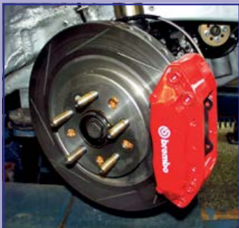
Škoda Octavia RS 2.0 TFSI - brake kit for front axle - parts Brembo Racing and Ferodo
