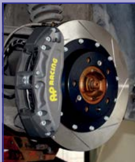
Porsche 911 996 - brake kit for both front and rear axles, parts AP Racing, Wilwood, Rensport
